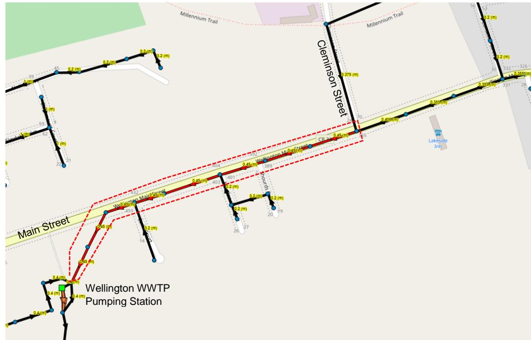
**Figure 3.3 – Main Street sewer upgrade to 450 mm (shown as red).**
